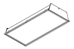
**RCFTB24 Recessed Lay-In for T-Bar Grid Ceiling**
