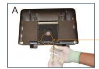
Uninstall the mounting bracket from fixture base plate by unscrewing the 2 hex socket studs.
