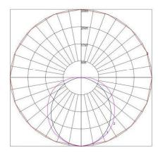
Maximum Candela = 3593 Located At Horizontal Angle = 0, Vertical Angle = 0
