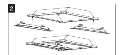
2. Insert the two brackets into the clearance between the housing and T-grid.
